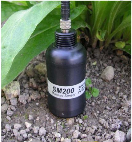
Example: Irrigate when SMC < 30% Inhibit irrigation when SMC > 40% Or Rainfall > 4 mm/h
