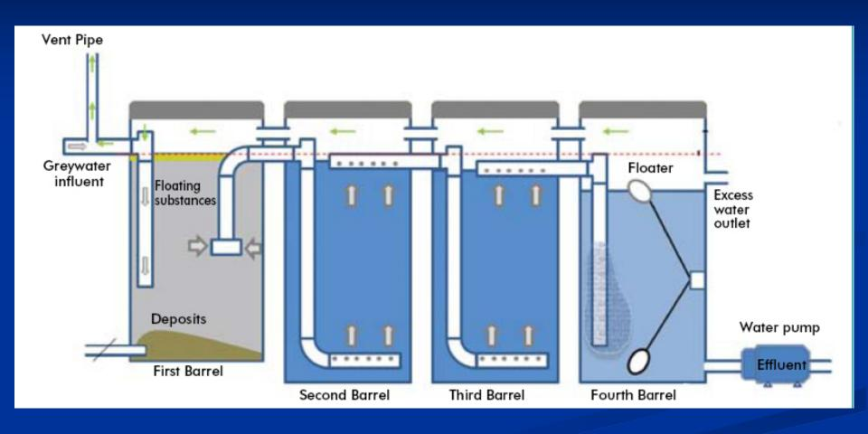
4-Barrel GW systems are watertight, airtight and odorless
